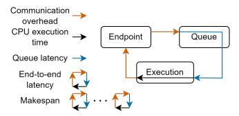
Figure 14: Differences in delay definitions
