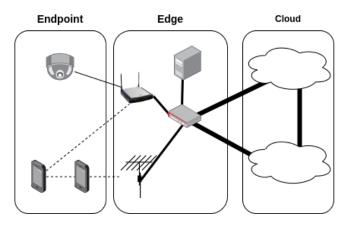
Figure 1: An overview of the compute continuum, showing that endpoints are owned by users, and the edge and cloud are owned by service providers inspired by [35]
