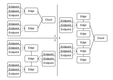
Figure 4: 3 potential system model edge setups, endpoints to edge to cloud, endpoints to edge cluster to cloud, and endpoints to edges to edges
