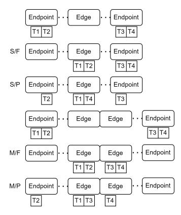
Figure 11: The 4 identified types of offloading
