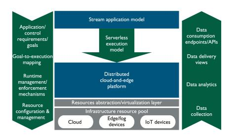
Figure 8.5: High level architecture of cloud and edge data analytics platform (6).
