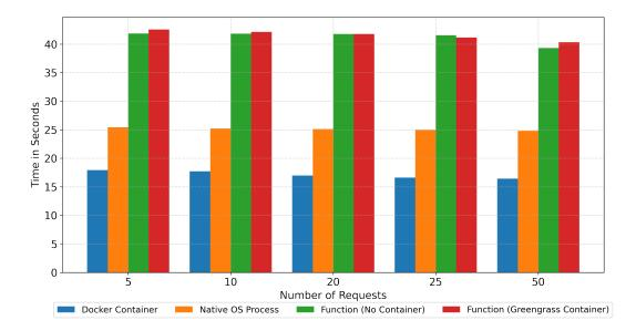
Figure 6.10: Total execution time for Edge Concurrent Workloads (W2) in 100 requests with several sensors -threads- (5, 10, 20, 25, 50) in four runtimes: Native OS process, Docker Container, Lambda (Greengrass and No Container).
