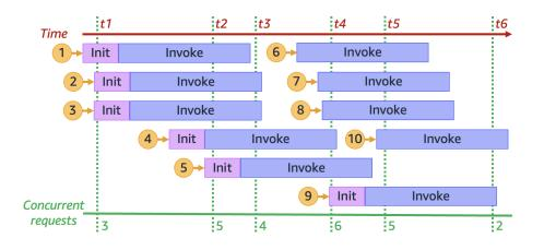
Figure 4.5: Concurrent executions with respect to the incoming requests, when multiple requests are done simultaneously with various execution environments working (10).
