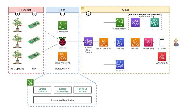
Figure 3.4: Components of Edgeless Ecosystem applied in Precise Agriculture.
