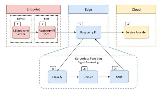
**Figure 3.3:** Design of Edgeless: serverless functions deployed at the edge for processing inflight data coming from microphone sensors.
