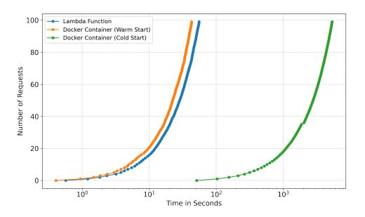
Figure 6.1: Total execution time for Cloud Sequential Workloads (W1) with 100 requests from three execution environments: 1. Lambda and Docker (2. cold start and 3. warm start).
