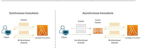
**Figure 4.6:** Lambda invocation methods: Synchronous, where a dedicated channel is established between the client and function. Asynchronous, where the client does not wait for a response from the function
