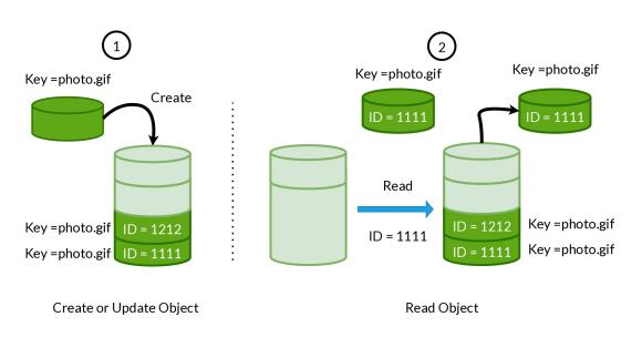
Figure 4.9: S3 versioning on bucket, on (1) create and update object and (2) read object.
