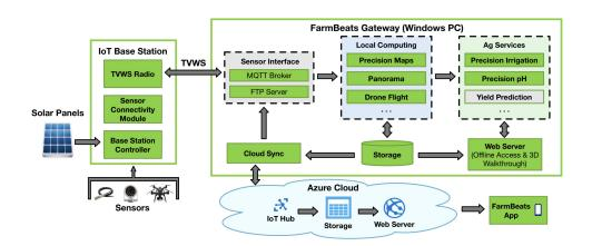
Figure 8.1: FarmBeats architecture for edge processing in drones and other IoT devices (1).
