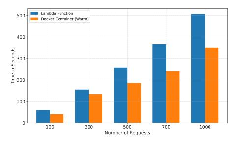
Figure 6.4: Total execution time for Cloud Sequential Workloads (W1) with several of requests (100, 300, 500, 700 and 1000) from two runtimes: Lambda and Docker containers (warm).
