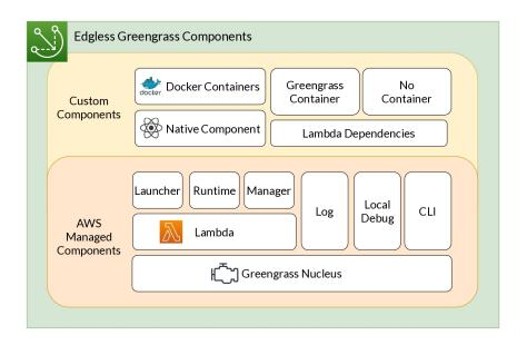
Figure 4.3: Greengrass core device component decomposition.
