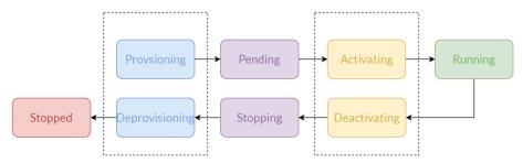
Figure 6.3: Process for scheduling a Docker container in ECS, taking on average between 50 and 60 seconds from the Provisioning phase to the Stopped phase.
