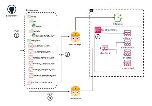
Figure 5.4: Deployment arrangement for cloud experiment setup using SAM
