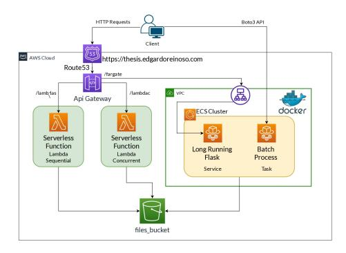
Figure 5.1: Setup for evaluating serverless performance in the cloud
