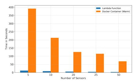
Figure 6.7: Total execution time for Cloud Concurrent Workloads (W2) in 100 requests with several sensors -threads- (5, 10, 20, 25, 50) using two runtime: Lambda and Docker containers (warm).
