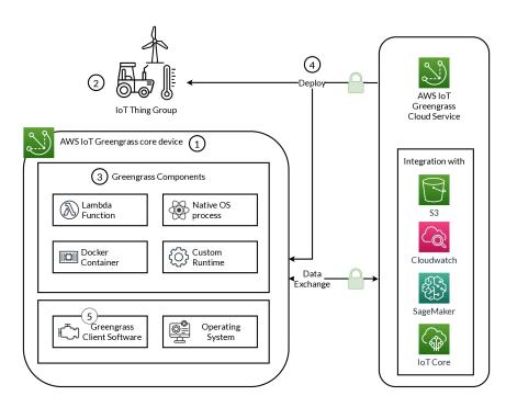
Figure 4.1: AWS IoT Greengrass device is composed by: (1) Core device, (2) Client device, (3) Greengrass Components, (4) Deployments, (5) Greengrass core software.
