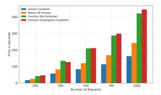
Figure 6.9: Total execution time for for Edge Sequential Workloads (W1) with several requests (100, 300, 500, 700 and 1000) in four runtimes: Native OS process, Docker Container, Lambda (Greengrass and No Container).
