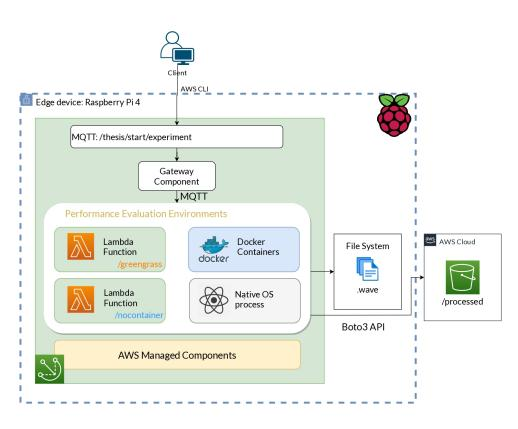
Figure 5.2: Setup for evaluating serverless performance at the edge
