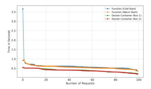
Figure 6.2: Time per execution for each individual request. 100 requests are executed twice by different runtimes, Lambda and Docker Containers. Furthermore, it is visible the dimension of cold start and how much of an impact it may have in the first execution request.
