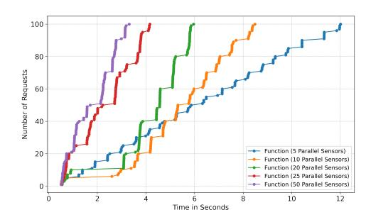
Figure 6.5: Total execution time for Cloud Concurrent Workloads (W2) in 100 requests with several sensors -threads- (5, 10, 20, 25, 50) invoking concurrent Lambda function.
